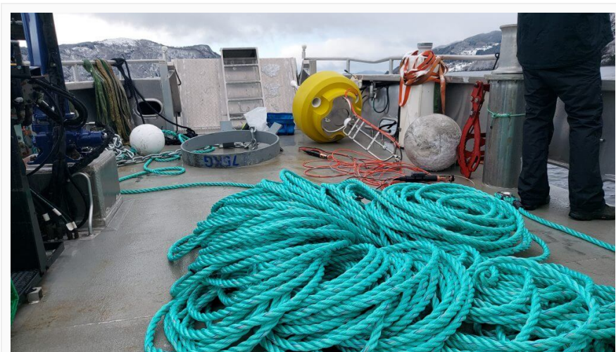
Figure 6: Buoy mooring hardware carefully arranged on deck to avoid tangling.
