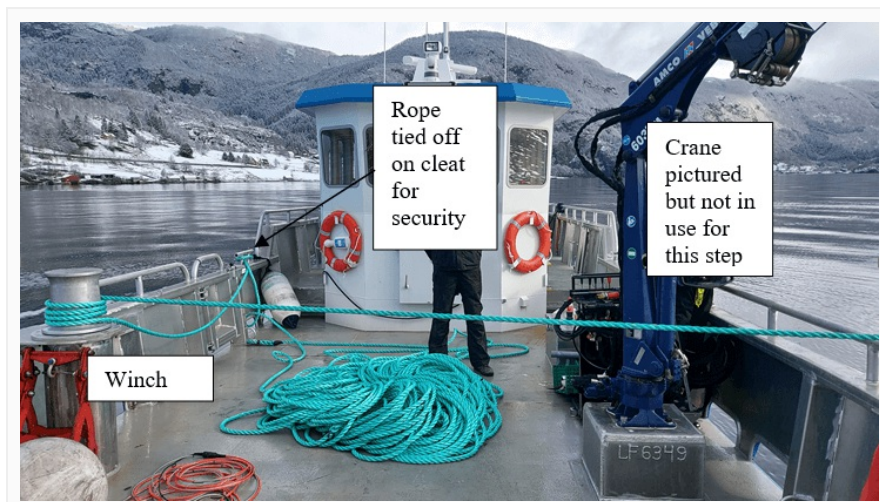
Figure 9: Paying out the mooring line using the winch.
