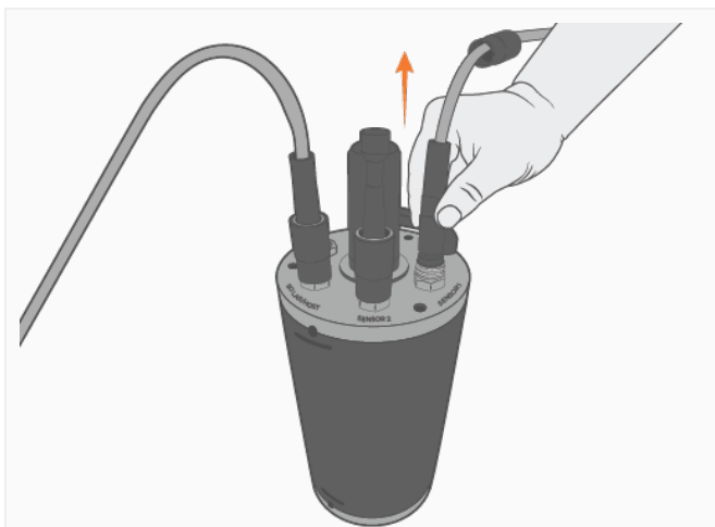
Figure 9: Proper disconnection of sensor cable with vertical removal.
