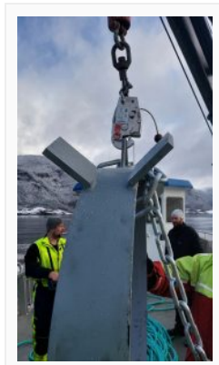
Figure 7: Anchor supported by off-load hook.
