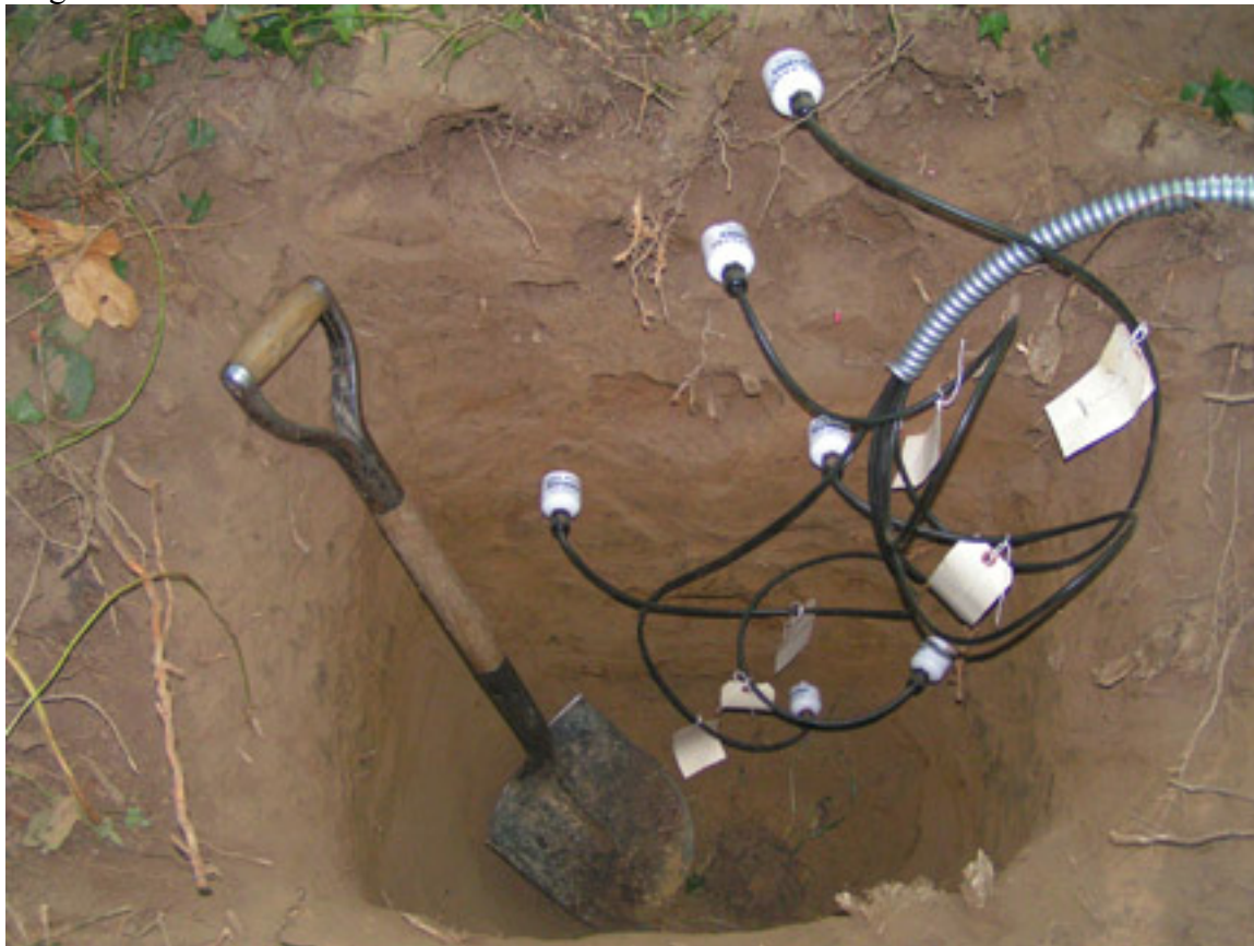
Figure 3.6 Six Hydra Probes installed into 6 distinct soil horizons.
