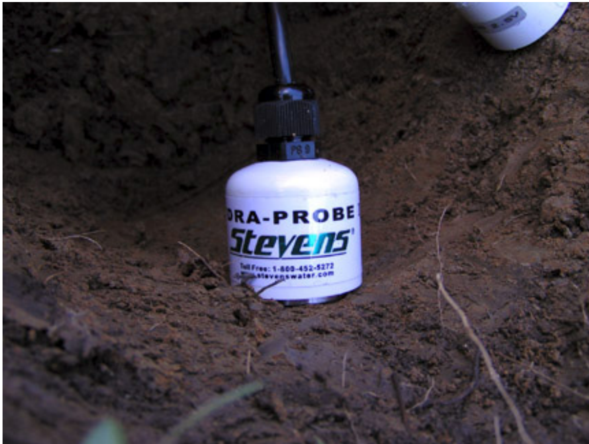
Figure 3.5 Hydra Probe Installed in undisturbed soil.
