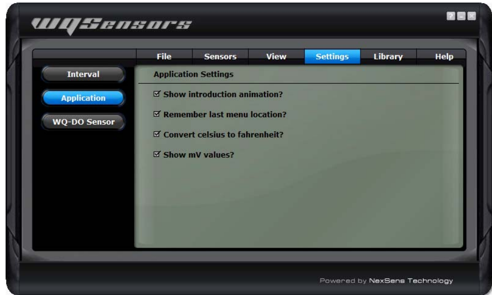
Figure 19: The Application Settings menu in the Settings tab in WQ Sensors software
