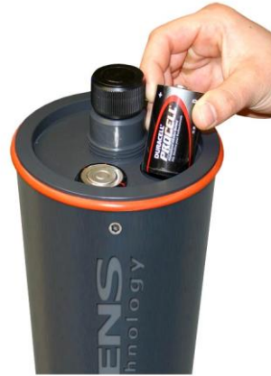
Figure 4: Installing batteries in the SDL500R
