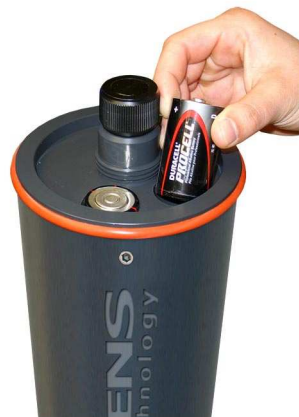
Figure 4: Installing batteries in the SDL500
