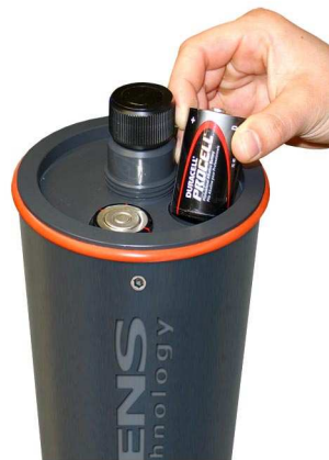
Figure 4: Installing batteries in the SDL500
