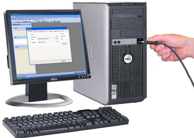
Figure 5: Connecting the SDL500 USB interface cable to a PC running iChart software
