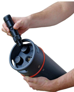
Figure 12: Connecting a T-Node temperature sensor to SDL500 sensor bulkhead
