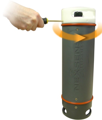
Figure 3: Unthreading the SDL500 battery lid from the communication bulkhead for battery installation
