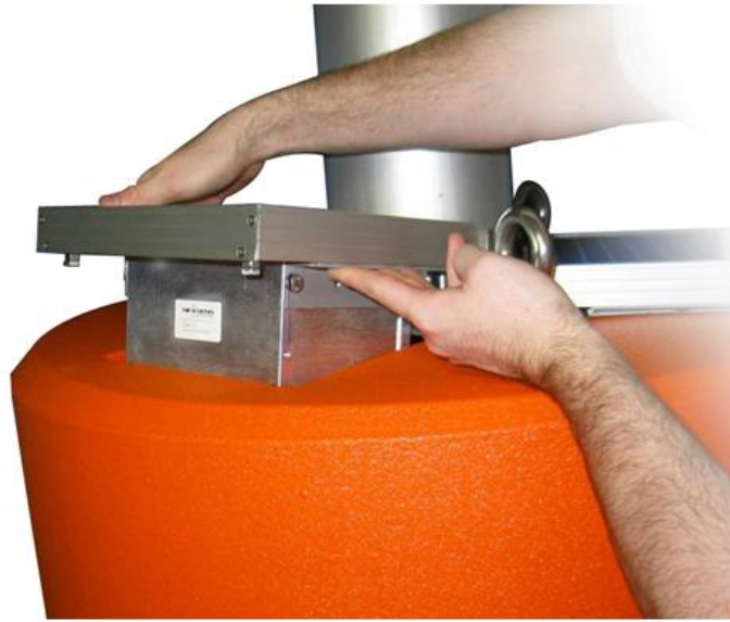
Figure 7: SP5 solar power pack installation
