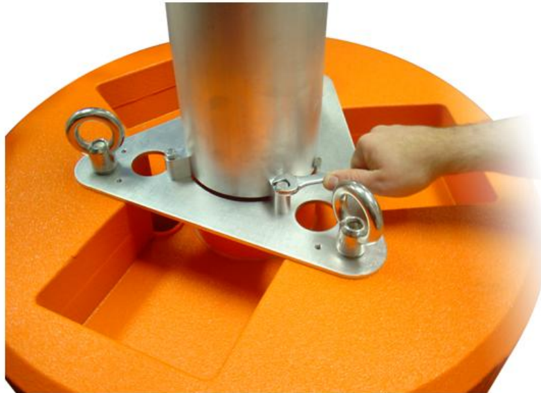
Figure 6: Tie down bolts are tightened to keep buoy tower from hinging back
