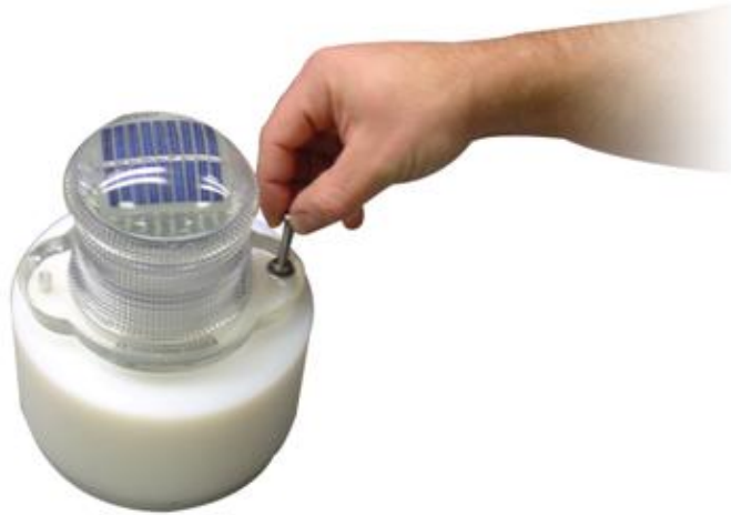
Figure 10: 1/4" hardware is used to fasten the beacon to the buoy tower lid Use the supplied screws ( \frac{1}{4} "-20 x \frac{3}{8} "") to mount the buoy lid with beacon to the top of the tower.
