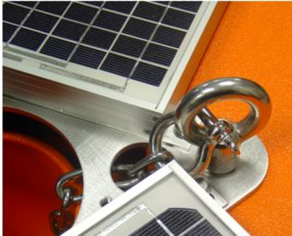
Figure 27: Buoy attachment chain connected to top side mooring eye
