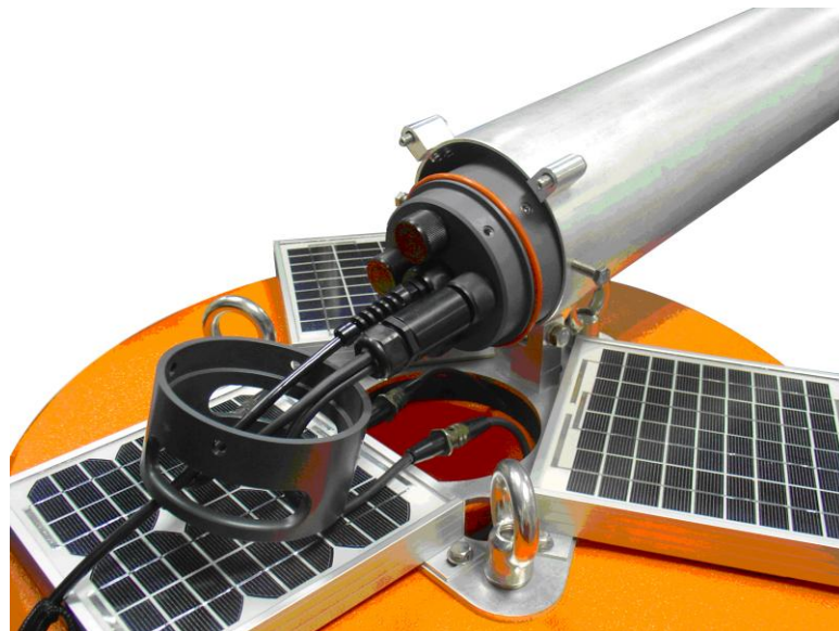
Figure 15: SDL500 positioned slightly out of tower with sensors connected Reconnect the guard to the SDL500 data logger.
