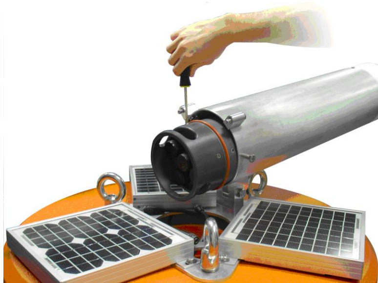
Figure 13: SDL500 positioned partially out of tower
