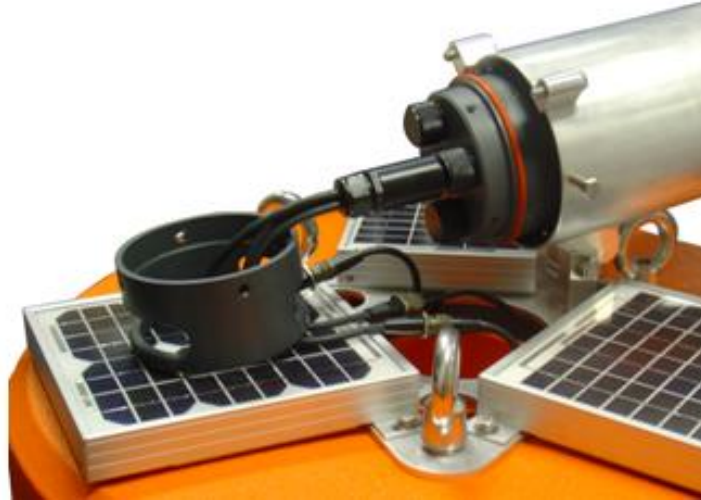
Figure 14: SDL500 positioned slightly out of tower with guard removed and power harness connect to port D
