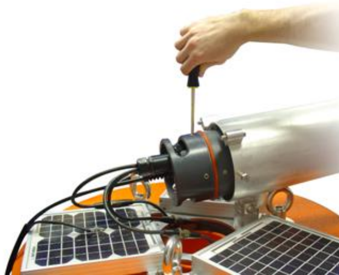
Figure 16: SDL500 positioned slightly out of tower with connections made to sensor bulkhead and guard re-installed
