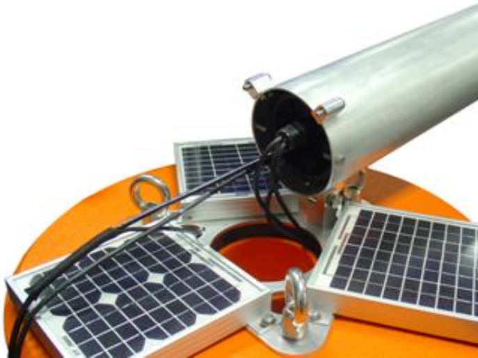
Figure 26: Underwater connections positioned outside of the buoy well
