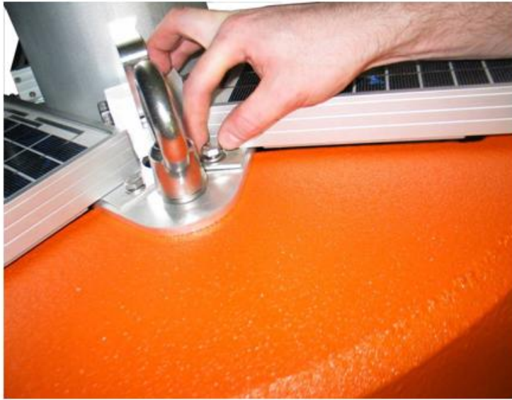
Figure 9: 5/16" hardware is used to fasten the solar power packs to the buoy top plate
