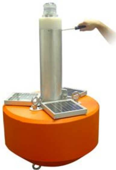
Figure 11: 1/4" hardware and 3/16" Allen wrench are used to tighten the buoy tower lid to the tower
