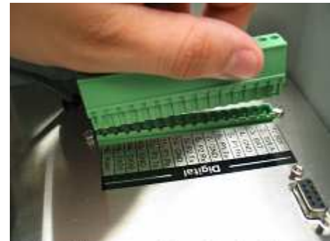
Note: the green terminal strip unplugs from the iSIC
